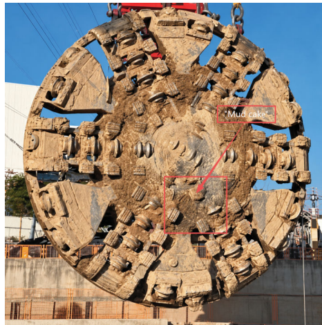
Figure 8 - “Mud-Cake” at Cutterhead (photo taken from other project)
