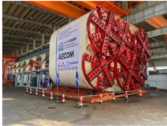
Figure 15 - RTBM Assembly for testing in fabrication yard before delivery to Hong Kong
